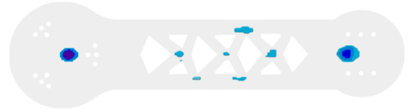
Figure 28: Top view of simulated pore distribution via MAGMASOFT.
